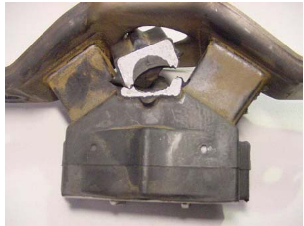
Gearbox support insulator
